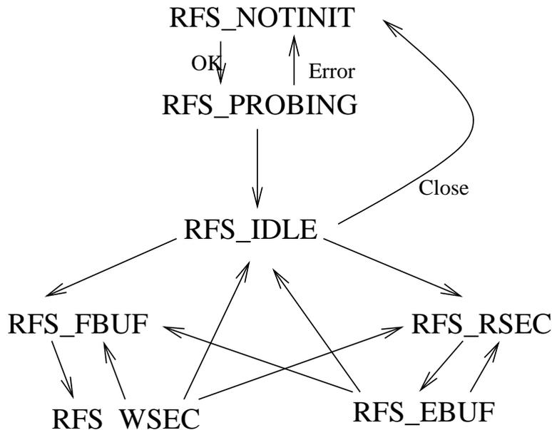
Figure 3: `rfc(4)`'s internal states.
